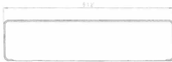
FIGURE 3—TREX® TRANSCEND® AND SELECT® 2X6 SQAURED-EDGE DECK BOARD PROFILE (See Sections 3.1.1 and 3.1.2 for Board Thickness)
