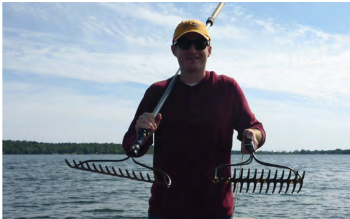
Figure 3. Two different rake samplers used during the Eagle Lake surveys. [left] Fixed head sampler. [right] Double headed throw rake.
